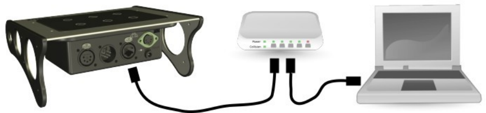
Figure 2: Patch cable HUB/Switch connection
