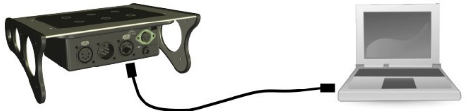
Figure 1: Cross cable direct connection
